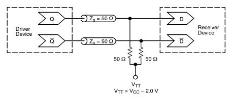
Figure 7. Typical Termination for Output Driver and Device Evaluation (See Application Note AND8020/D – Termination of ECL Logic Devices.)
