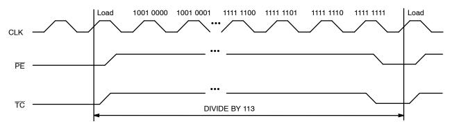
Figure 5. Divide by 113 EP016A Programmable Divider Waveforms
