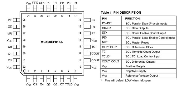
Warning: All  $V_{CC}$  and  $V_{EE}$  pins must be externally connected to Power Supply to guarantee proper operation.
