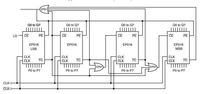
Figure 6. 32-Bit Cascaded EP016A Programmable Divider
