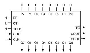
Figure 4. Mod 2 to 256 Programmable Divider
