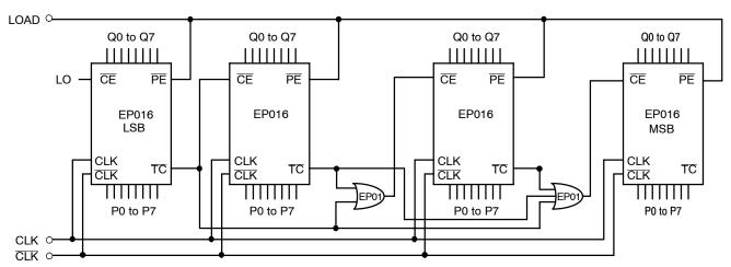
Figure 3. 32-Bit Cascaded EP016A Counter
